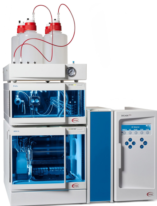
Figure 5: Recommended instrument configuration for this application: the ALEXYS Carbohydrate Analyzer with Solvent Switch Valve. The system consists of a P6.1L pump with integrated degasser and Solvent Switch Valve (SSV) for the option to run step gradients, an AS6.1L autosampler, an ET 210 Eluent tray for helium blanketing, and the DECADE Elite electrochemical detector. A CT 2.1 column oven with broad temperature range can be added optionally for separations under near-ambient temperatures. The ALEXYS Carbohydrate Analyzer can be operated under different Chromatography Data System (CDS) software: DataApex™ Clarity™ CDS (version 8.3 and up) or Thermo Scientific™ Chromeleon™ CDS (version 7.2 SR 5 and up).
